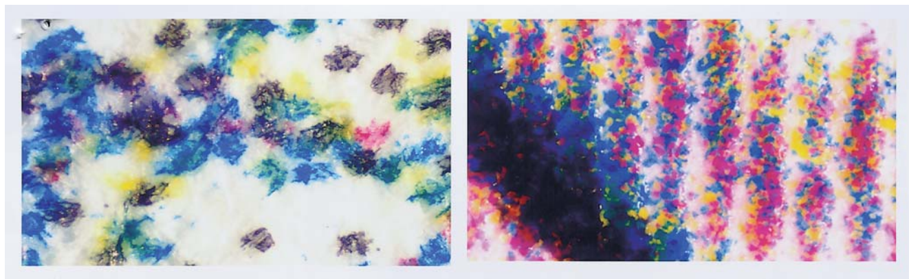
FIG. 1—Comparison of documents produced using color inkjet printing (left) and toner (right) at 40× magnification.
